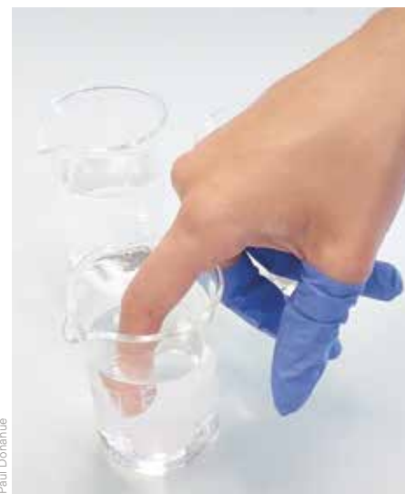
Photo: Virus transfer experiments using bacteriophage MS2 (enteric virus surrogate).
