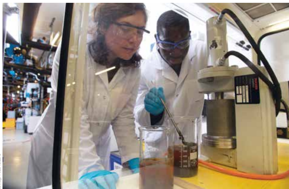
Photo 2: PhD students Stanley Sam and BJ Ward measure dewatering performance of faecal sludge using a bench-scale Bucher filter press.
