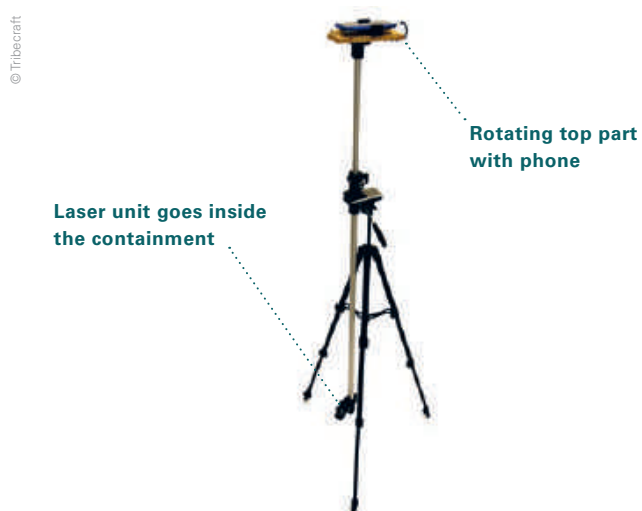
Photo 2: The Volaser prototype set-up with the tripod, top part and laser.
