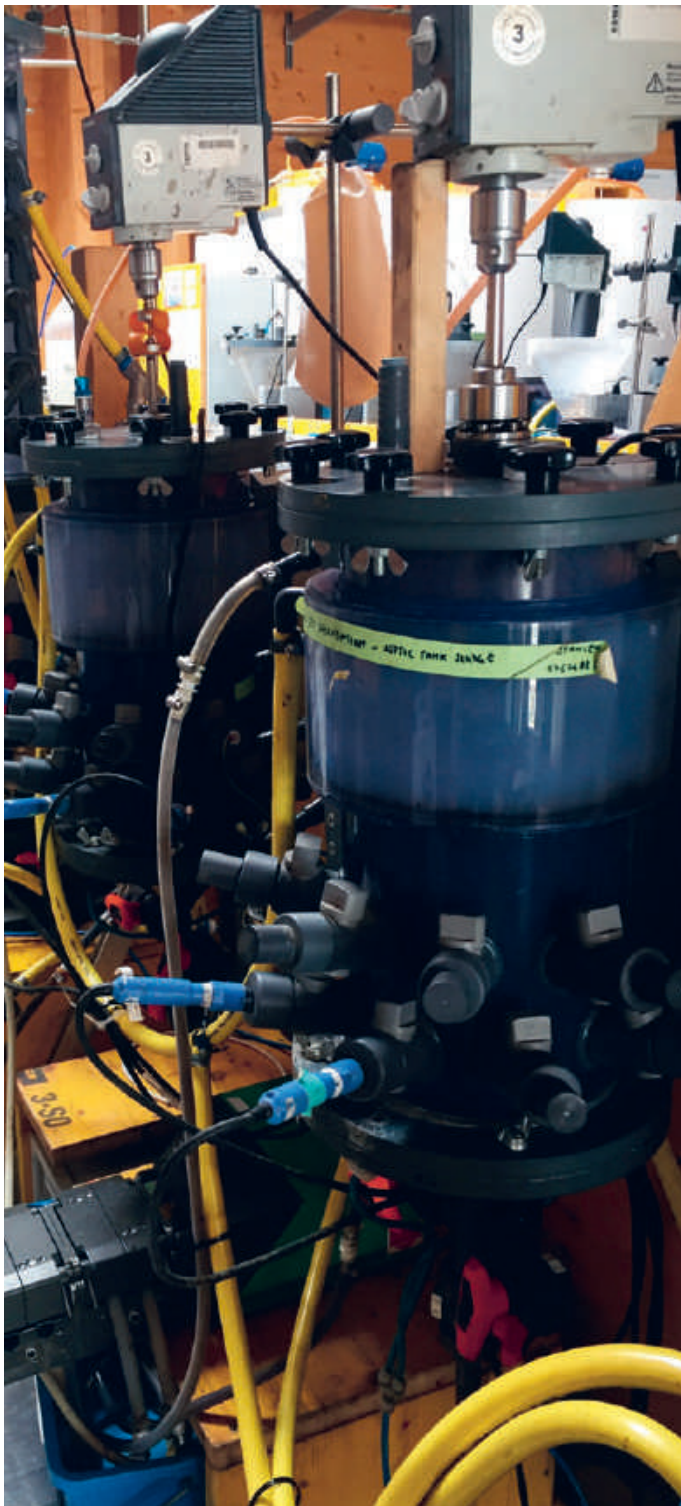
Photo 2: Reactors running controlled digestion experiments to mimic storage in onsite containments.
