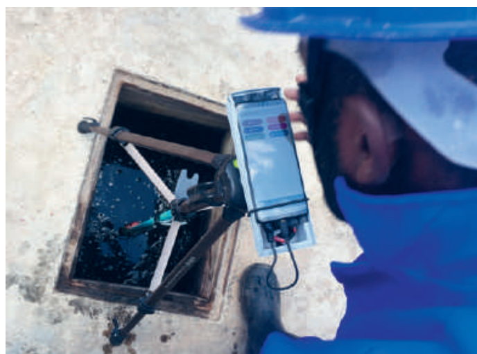
Photo 1: Using the Volaser with the smartphone app in a septic tank in Lusaka, Zambia.
