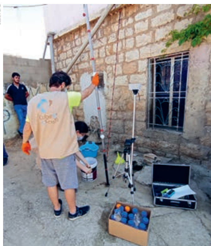
Photo: Sampling team from CubeX taking faecal sludge samples from an onsite sanitation containment in Lebanon with the Volaser and a core sampler.
