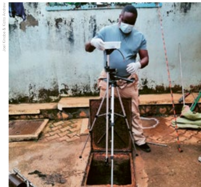
Photo: Measuring fecal sludge volume with a Volaser in a septic tank in Uganda.
