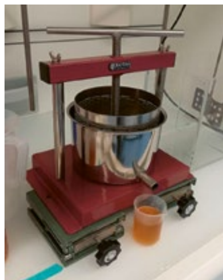
Photo 2: Fruit press tested to dewater conditioned faecal sludge.
