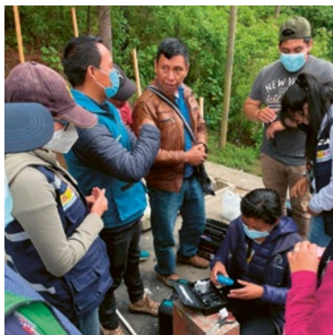
Photo 2: Measuring free residual chlorine concentration after installation of the chlorinator in collaboration with water committee members, the Health Ministry, the Municipality and Helvetas Guatemala.
