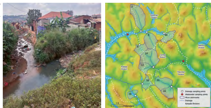
Photos: Left: Drainage channels in Kampala, Uganda; Right: Ten drainage sampling points (white circle) with the corresponding micro-catchments (grey region) and two wastewater sampling points at centralised treatment plants (red circle) across five divisions of Kampala.
