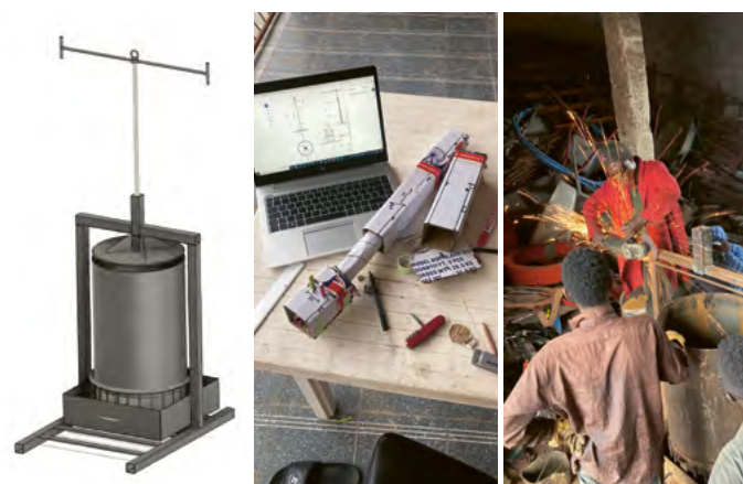
Figure 2: From 3D-drawing, to 3D-mockup, to manufacturing of the press in Freetown (left to right).
