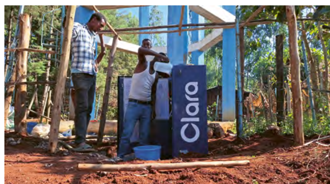
Photo: Operator refilling Clara V2 with brine solution.
