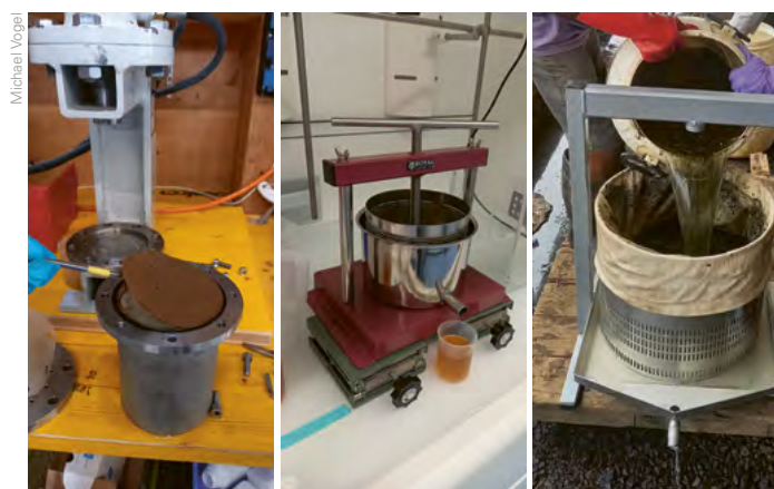
Figure 1: Laboratory filter press (left), commercially available fruit presses with a volume of 3L in the laboratory (centre) and 50L at Kingtom FSTP (right).
