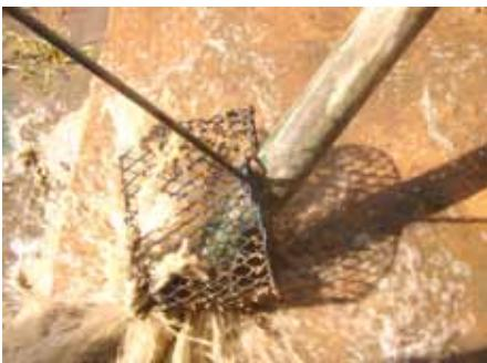
Photo 5: Manual and mobile screening grid.
