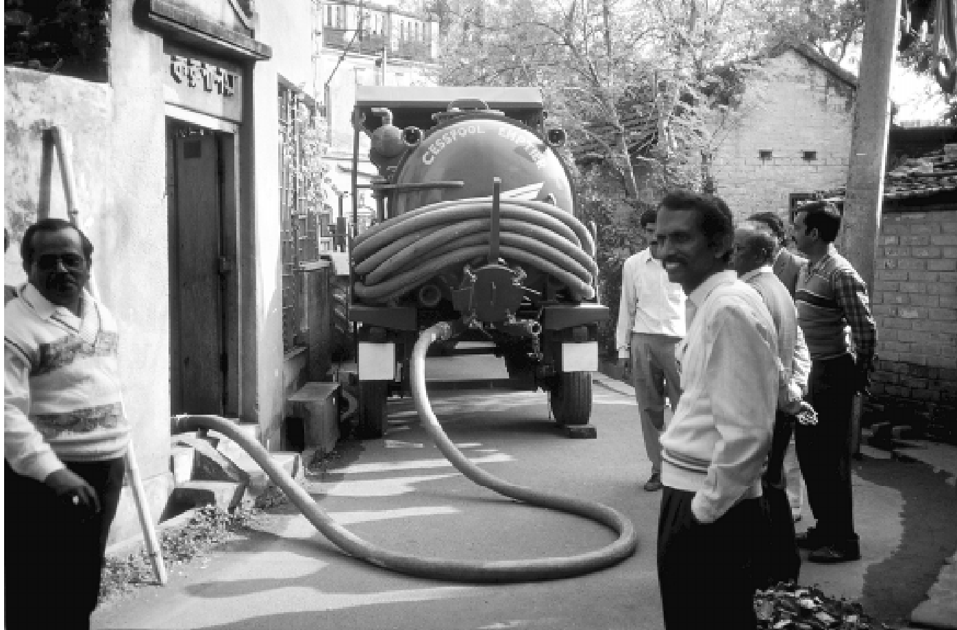
Fig. 1 Septage collection with a 2-m 3 cesspool emptier in a side lane in Bharakpur, West Bengal, India. Hauling small volumes of FS over long distances in metropolitan areas is uneconomical. Sustainable strategies involving semi-centralised treatment must, therefore, be developed
