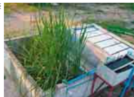
Photo 1: Pilot-scale experimental setup with constructed wetland, sand filter and anaerobic filter (left to right) at AIT, Bangkok, Thailand.
