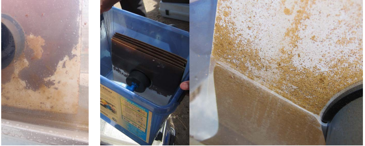
Figure 41 Pictures of the membranes showing sloughing of the biofilm after 3-6 month of operation (Photos: M.Peter, S.Derksen)
