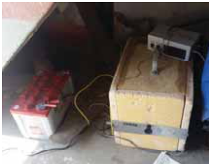
Figure 7 Incubator connected to solar-panel / battery system
