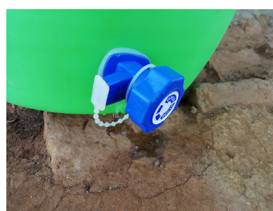
(b) Leaking tap
