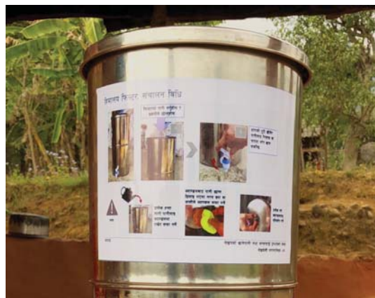
FIGURE 2.6: Manual with OM aspects in Nepalese on a MCC filter in the field.
