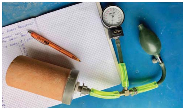
FIGURE 2.7: Adapted blood pressure measurement device to assess the air flow resistance of the MCC candles.
