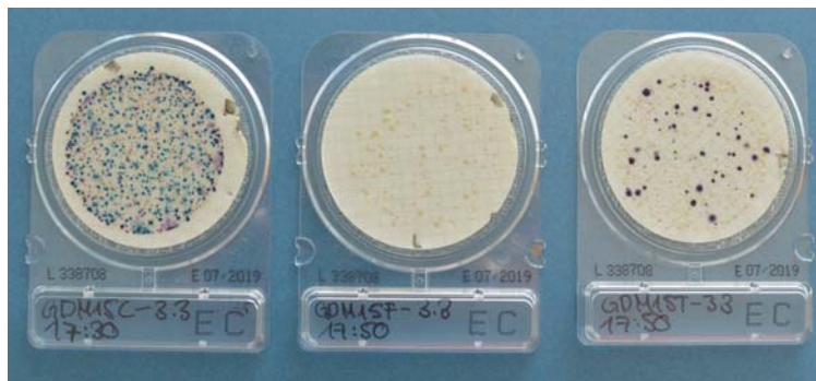
FIGURE 3.13: EC plates from the raw water, filtered I and filtered II (left to right) from a GDM filter with recontamination or regrowth in the storage.
