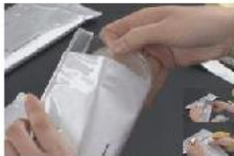
Take out a set of 4 plates. ( Do take care to handle the plates and keep the pouch sealed to avoid a quality loss from light and moisture. )
