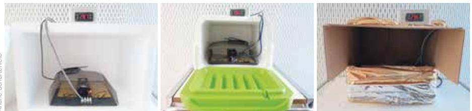
Photo: Incubator shells tested. Polystyrene foam box (left), hard plastic cooler box (middle), and cardboard box covered with a survival blanket (right).
