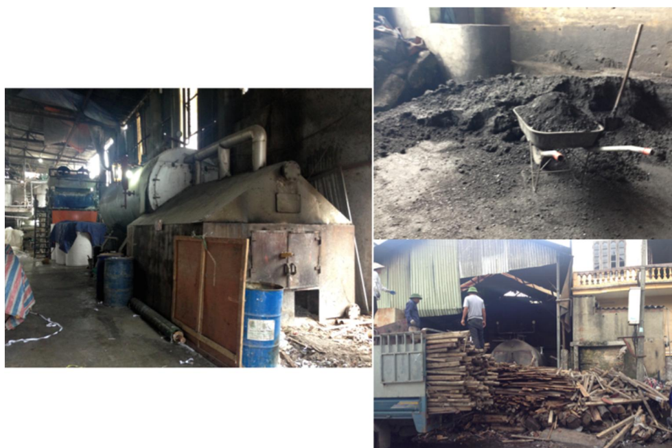
Figure 9: Steam generator in recycled paper production using coal or wood
