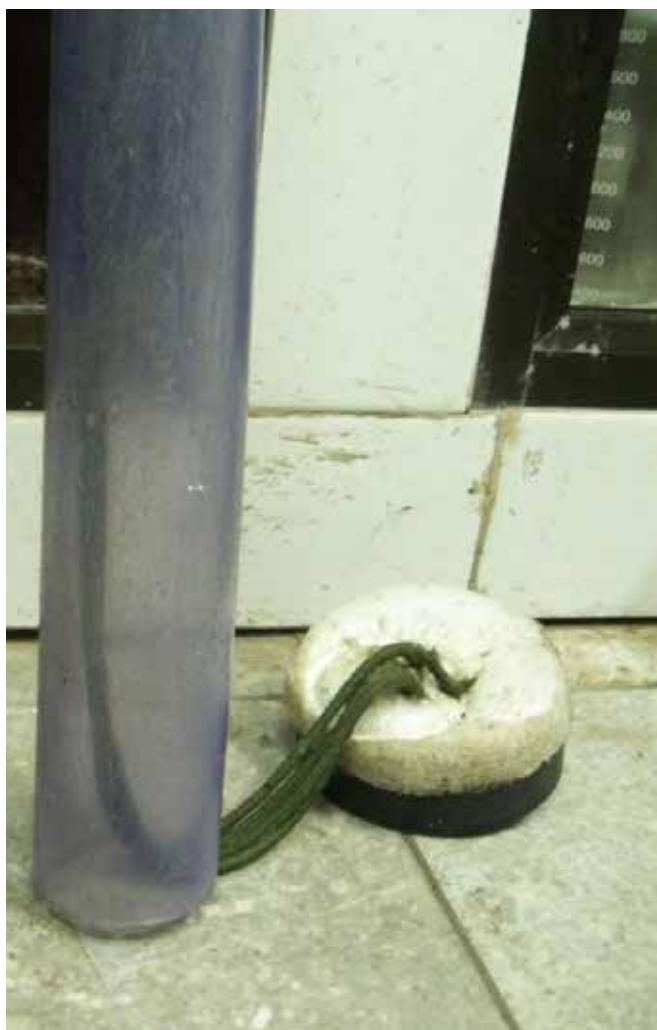
Figure 2: Bottom of the core sampling device
