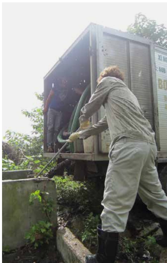
Figure 3: Sampling with a bucket mounted on a bar
