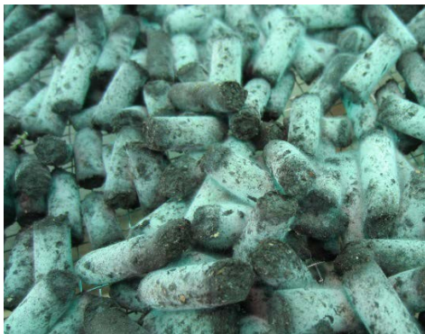
Figure 11: Mold formed during drying on FS pellets co-pelletized with spent grain.
