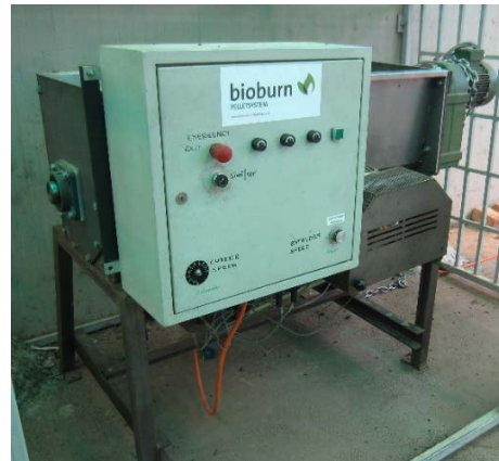
Figure 2: Bioburn pelletizer installed at NWSC Lubigi
