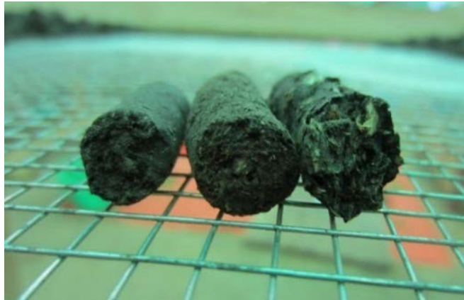
Figure 10: Compactness of three different pellets. The score (see Table 2) decreases from the left (score 3), to the right (score 2).
