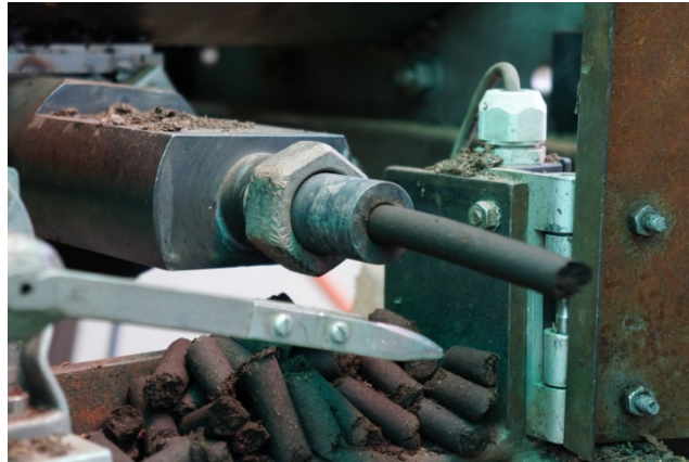
Figure 8: Pellet leaving the extruder through the nozzle.
