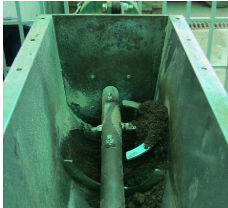
Figure 7: Rotating shovels pushing the FS and biowaste mixture into the extruder.
