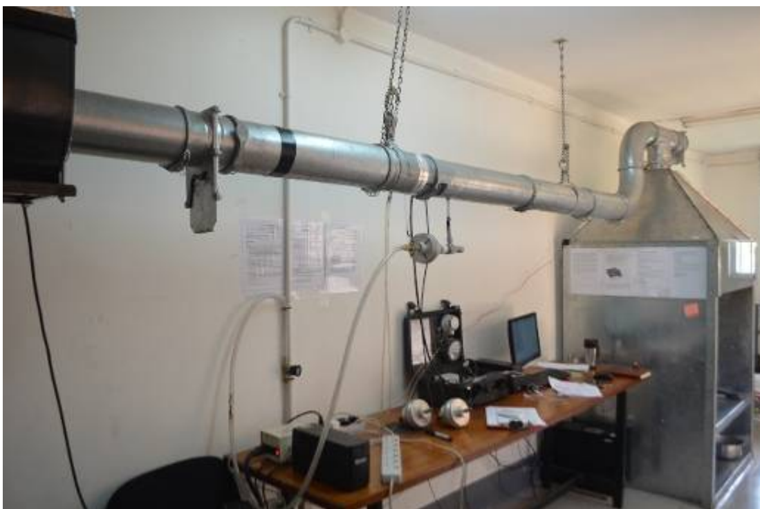
Fig 5: LEMS set up with the gravimetric system for emissions measurement PM2.5
