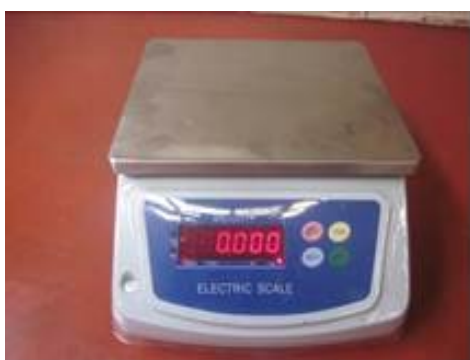
Fig 4: 30 kg digital weighing scale, used during the WBT
