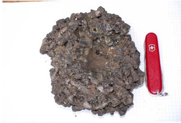
Figure 4.1: Clinker formed during an experiment with FS
