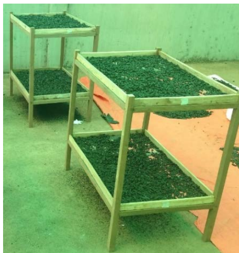
Figure 4: Faecal sludge drying with drying racks
