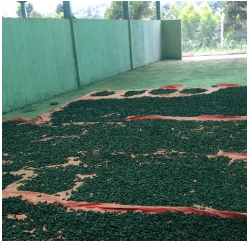
Figure 1: Drying of faecal sludge on tarpaulins.
