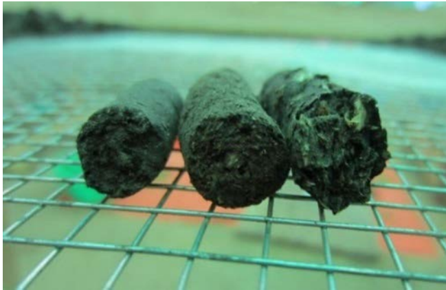
Figure 7: Compactness, texture of three different pellets.
