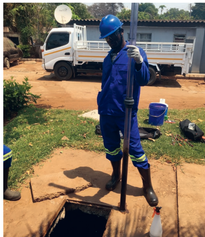
A core sampler is being used to take a sample from a septic tank in Lusaka.
