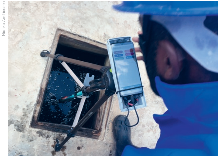
Photo 1: Using the Volaser with the smartphone app in a septic tank in Lusaka, Zambia.
