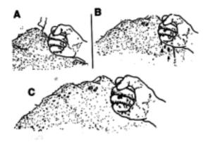
Figure 7.4: Testing of Moisture Content: Protect your hand with a glove. Take a handful of compost and squeeze it in your fist. A: If no water is squeezed out, the compost is too dry; **B**: If many drops can be squeezed out, the compost is too wet; **C**: If few drops can be squeezed out, the moisture content is ideal (CPIS, 1993)
