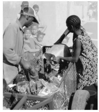
Photograph 5.1: The manual handcart with a grid container and broad wheels was adapted to the local sandy road conditions and high sand fraction. The sand falls through the grid, thus reducing the weight of waste (AGRESU – GTZ GmbH, Maputo, Mozambique)
