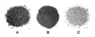
Photograph 8.1: A: Mature compost, B: ground compost and C: amended/ granulated compost
