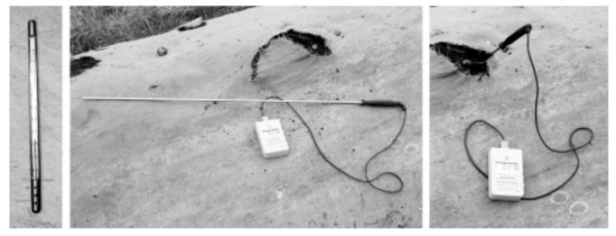
Photograph 7.10 - 7.11: Two types of thermometers: Alcohol thermometer and electronic thermometer with stick probe (Sandec, Switzerland)
