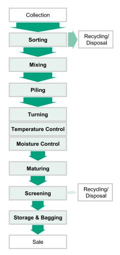
Figure 7.1: Flow chart showing composting process steps and material flows
