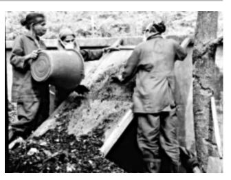
Photograph 7.14: Manual flat frame sieve (0.8 m x 1.4 m) on which workers 'rub' the compost through a wire mesh (5 mm mesh size). (Waste Concern, Bangladesh)
