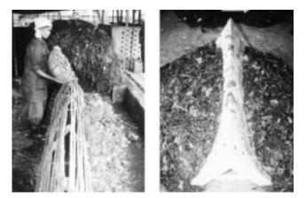
Photograph 7.4 and 7.5: The waste is piled around and onto the aerator (height 1.5 m) (Waste Concern, Bangladesh)
