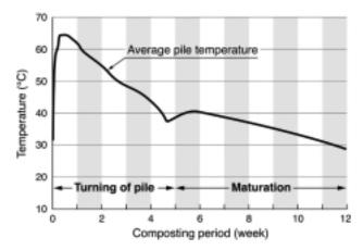
Figure 7.3: Temperature curve showing the two composting phases: thermophilic phase with frequent turning, maturation (mesophilic) phase with occasional turning
