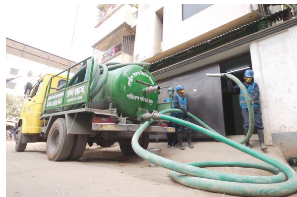
Figure 15: SWEEP vacuum tanker in operation in Dhaka
