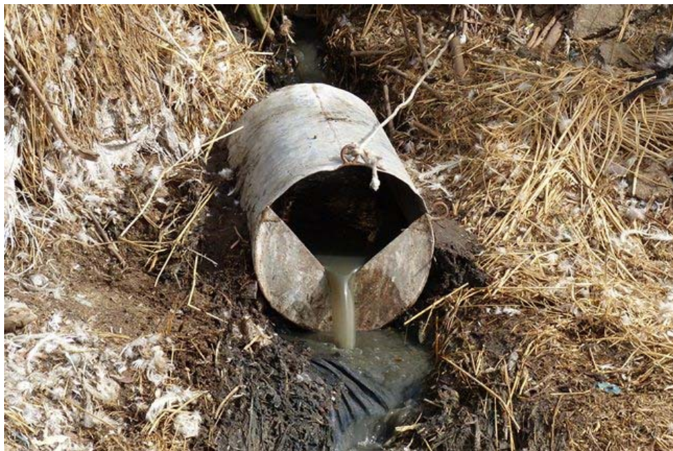
Flow measurement with a self-constructed weir, equipped with a data logger
