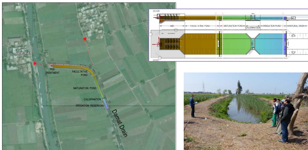
Figure 5: Example of the beginning of a drain converted into waste stabilisation ponds in series (Sources: Figures from ISSIP PM/TA, Memorandum, Feb. 2013 – Picture from Ph. Reymond, Beheira)
