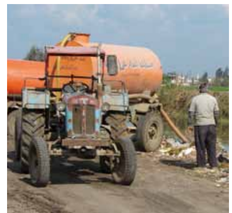
Photo 3: Wastewater and sludge pumped out of the traditional on-site facilities are dumped into the nearest canals or drains.
