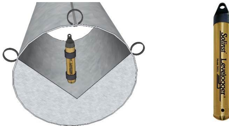
Figure 2: “KaCo” weir for flow measurement constructed by Eawag team; the datalogger is a Levelogger Gold model 3001, manufactured by the Solinst Company
