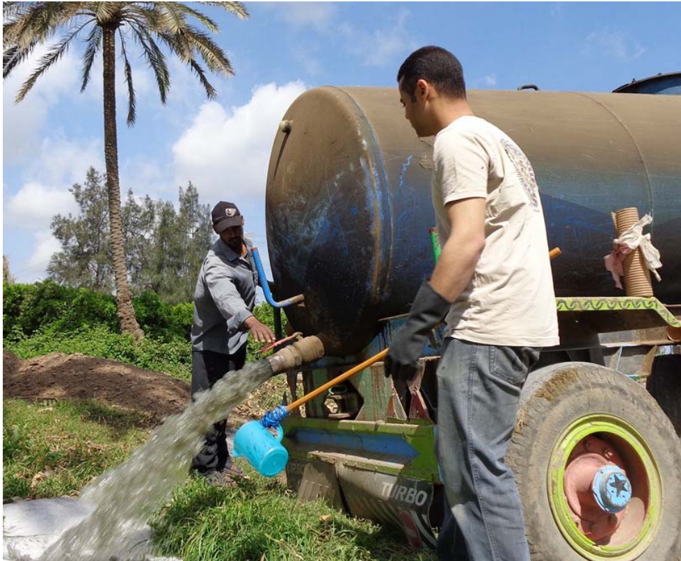
Figure 4: Septage sampling from a vacuum truck
