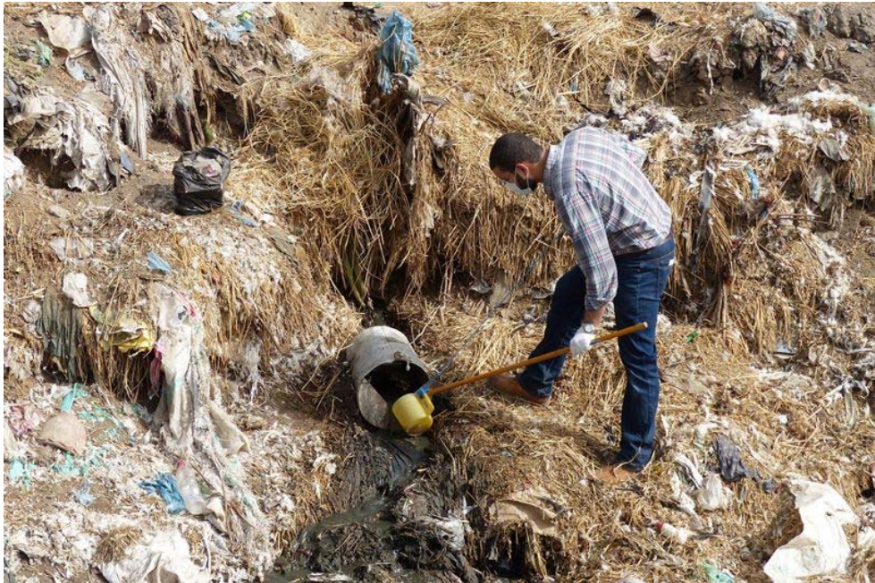
Figure 3: Raw wastewater sampling at the outlet of the flow measurement weir (in Fisha el Safra)
