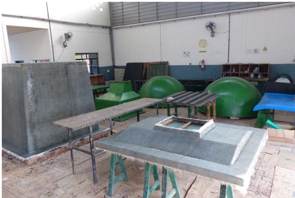
Small factory for prefabricated anaerobic treatment components in fibre glass, Bangalore, India (CDD Society, BORDA DEWATS)
