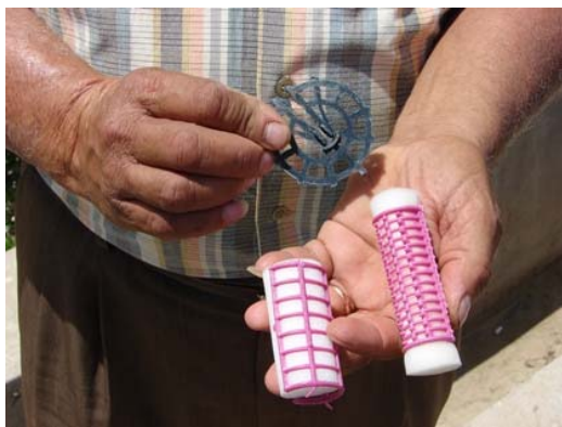
Different filter media: plastic chips found on the Egyptian market (top) and sponges in plastic frame (down)
