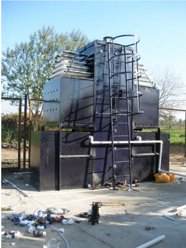
Left: the compact anaerobic tower; below: the pilot in Zenein WWTP, Giza, visited on 18.09.2011
