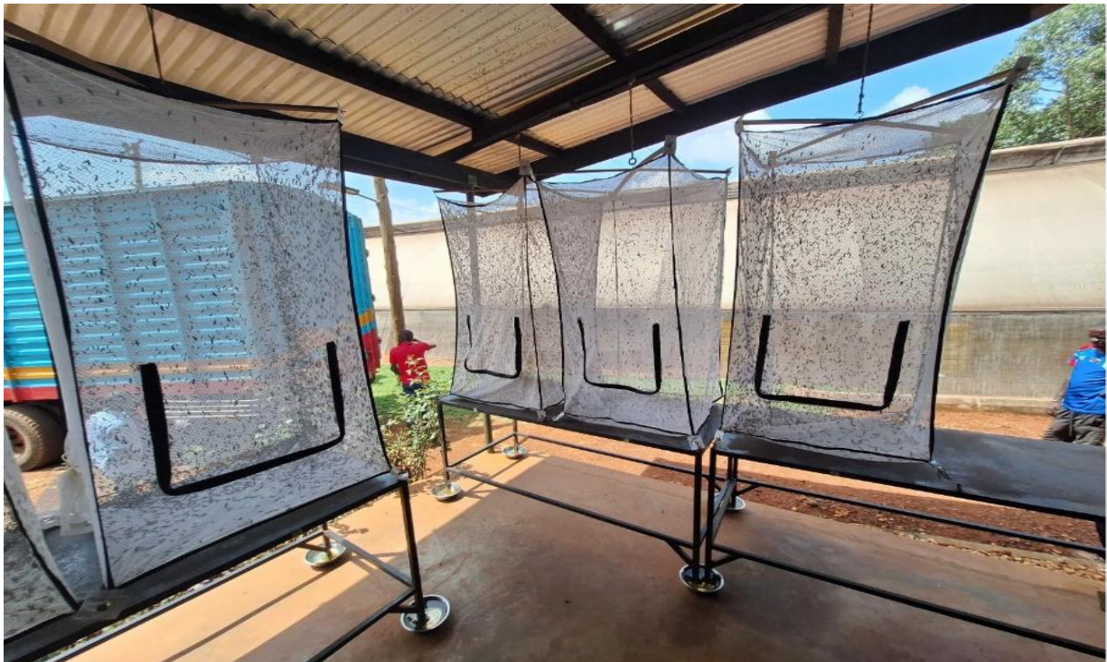
Figure 4-2: Bioconvision BSF plant - BSF "Love Cage" for the production of BSF eggs
