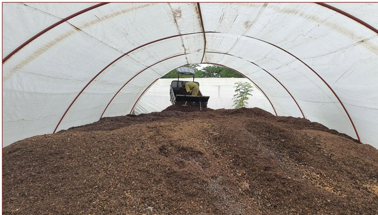
Figure 4-4: Chanzi BSF plant - Composting of BSF frass for further use as organic fertilizer
