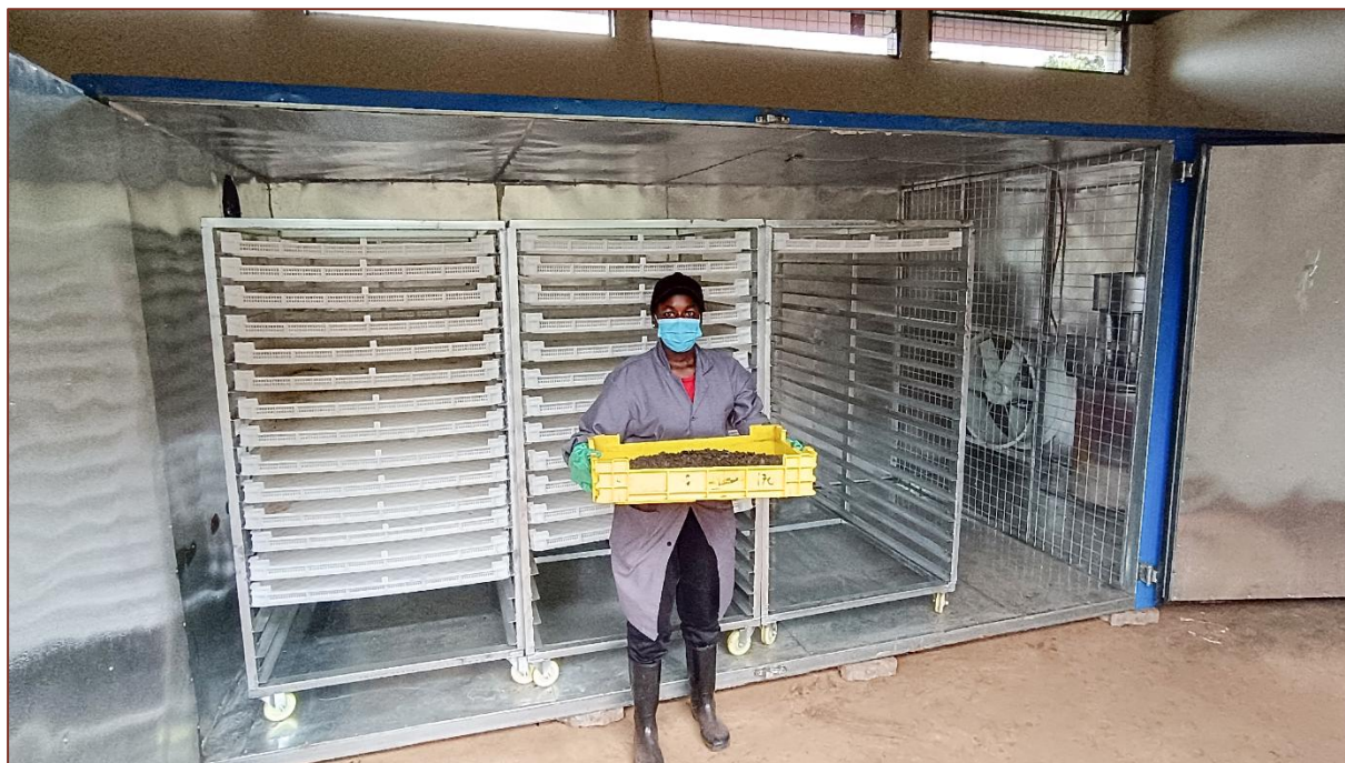
Figure 4-7: Alpha Protein Feeds BSF Plant - Trays for BSF rearing
