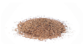
Washed beach sand Particle size: 0.8-1.5 mm
