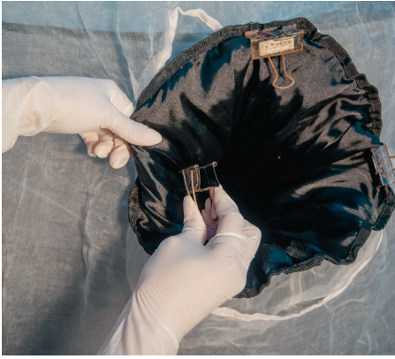
Step 2: Attaching dark cage to love cage from inside
