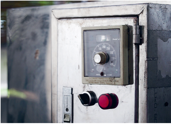
Step 1: Setting the thermostat to 65°C.
