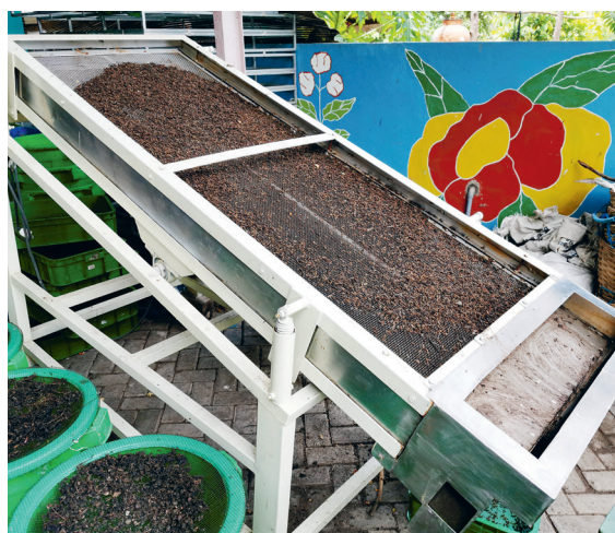
Figure 4–7: Shaking sieve to separate larvae from dry residue
