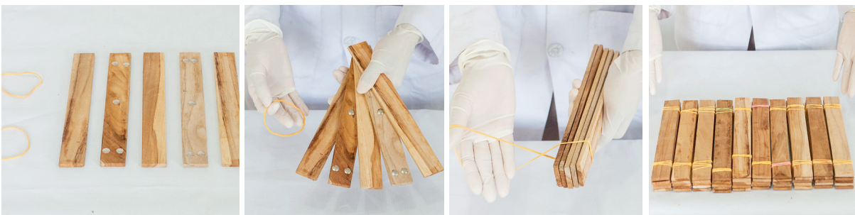
Step 6: Wooden sheets with pushpins to create a gap, allowing space for egg packages. The eggies are held together with two rubber bands
