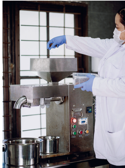
Step 2: Adding little by little dried larvae to the hopper.
