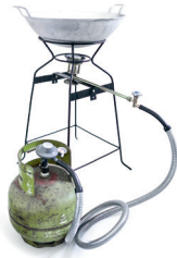
Wok pan setup Diameter pan: 30 cm Capacity: 3 kg/h
