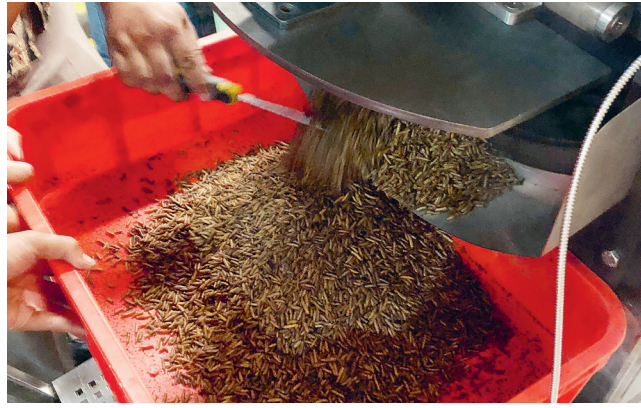
Step 3: Emptying drum via front flap door.
