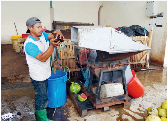
Step 3: Reducing particle size of biowaste by shredding the material
