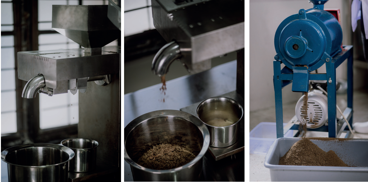
Figure 3: Screw pressing of BSFL (A) into press cake and press liquid (B) and further grinding of press cake into BSFL protein meal (C).
