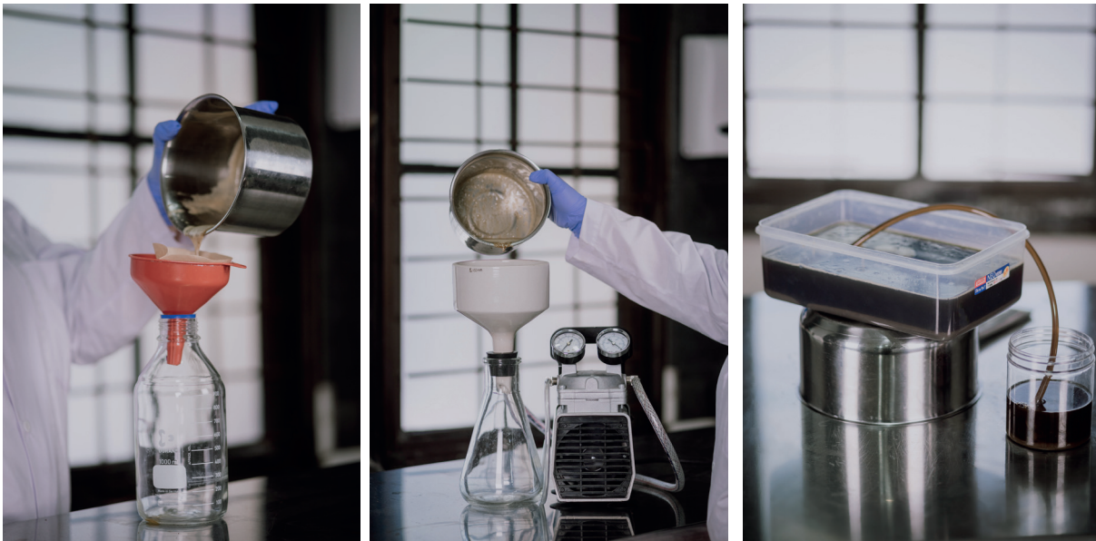
Figure 4: Oil refining options: A) Passive filtration set up, B) Filtration set up using a vacuum pump, C) Decanting set up
