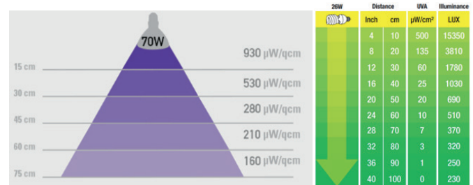
Figure 2: Light power of the SolarRaptor 70W spot lamp (left, ECONLUX GmbH) and the ExoTerra Natural light 26W lamp (right, Rolf C. Hagen Inc.)
