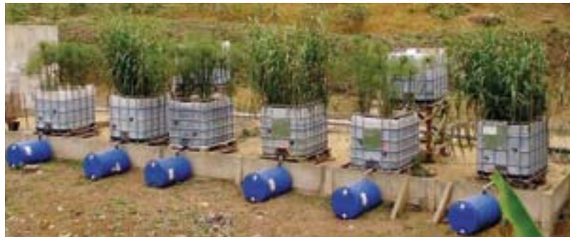
Vertical flow constructed wetland pilot bed for faecal sludge dewatering and mineralization in sub-Saharan countries.
