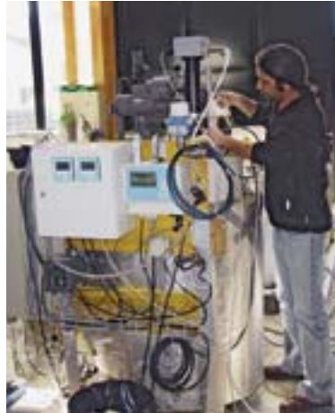
The 400-litre SBR reactor at the Eawag testing facility.
