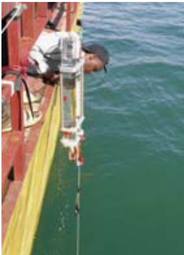
Sediment traps collect sinking algae – one of the factors in the lake's nutrient cycles.
