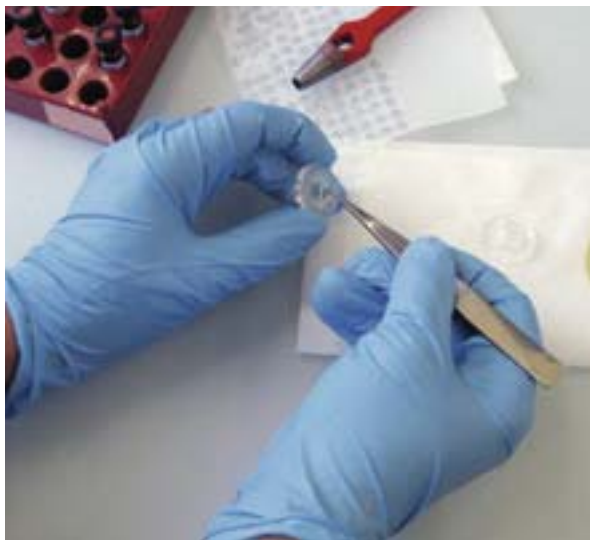
The stir disc is placed in one half of the glass cell. The entire glass cell, with the PDMS membrane in the middle, is then mounted on a magnetic stirrer in which the discs are not just rotated but tumbled end-over-end. This ensures that only a wafer-thin water layer remains unstirred at the gill membrane.
