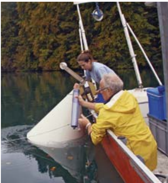
Retrieving methane traps – inverted funnels which capture the gas as it rises through the lake.
