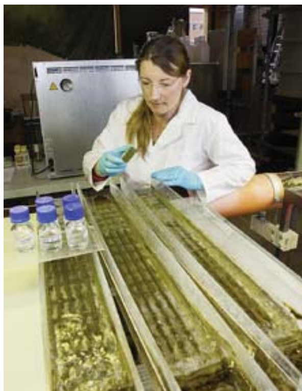
Flow-through channels are used to study the effects of various risk factors on algae.
