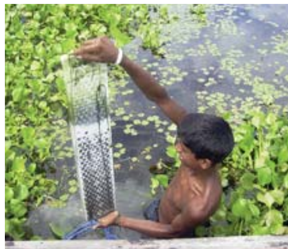
In a flooded paddy, a boy from Bashailbhog village (Bangladesh) helps researchers to collect porewater samples from various sediment depths.
