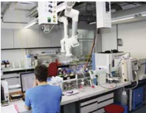
Top: Laying the foundations for the concrete stabilization elements designed to ensure earthquake resistance. Bottom: A modernized lab, now including a service column and local extraction units.
