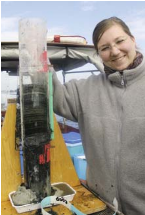
Nora Brede with a Greifensee sediment core. Thanks to the readily detectable annual laminations, eggs deposited in the sediment can be precisely dated.
