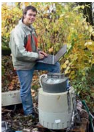
A researcher checks the automatic sampling process on the Petite Glâne river in the Lake Murten catchment.
