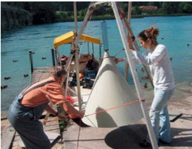
Researchers deploying funnel-shaped gas traps to study methane bubbles rising to the surface of Lake Wohlen.
