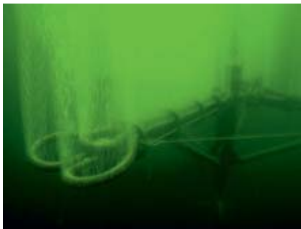
In 2009, diffusers released around 26 tonnes of oxygen into Lake Greifen.
