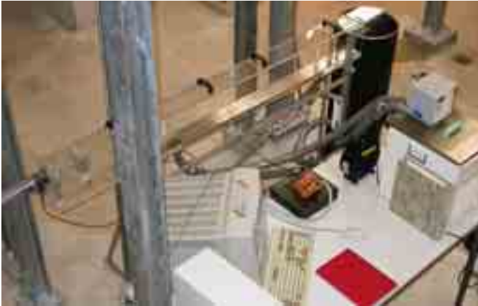
Fig. 2. The laboratory test rig, on which the effect of biofilm formation on heat exchanger efficiency was tested.
