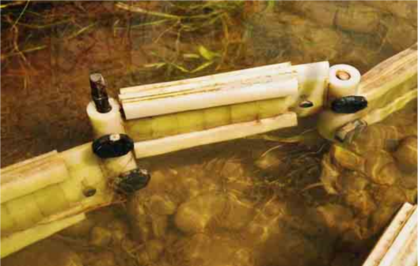
The sampling system in the Furtbach. The algal biofilms grow on glass plates.
