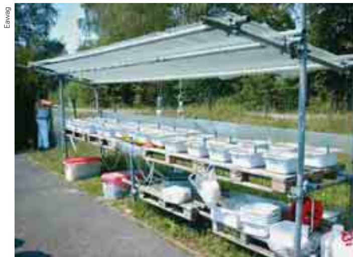
Fig. 1: Microcosm installation, in which natural algal biofilms are grown and exposed to elevated metal concentrations.
