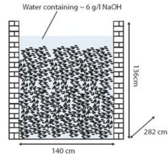
*Flushing of residual NaOH and reducing color - washing with water*
