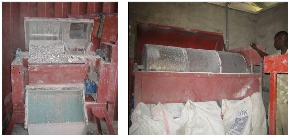
**Figure 8-3:** Crushing machine with attached sieving units and a separate sieving machine to facilitate and accelerate the sieving process.
