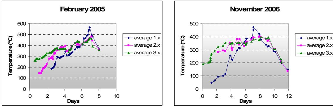
**Figure 2-3:** Temperature curves for charring batches carried out in February 2005 and October 2006. The blue line shows the temperature in the bottom, the purple line the temperature in the middle and the green line the temperature in the top layer of the bone char.
