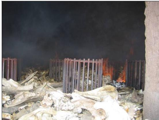
**Figure 2-2:** Storage of the bones and the charring process at its beginning.
