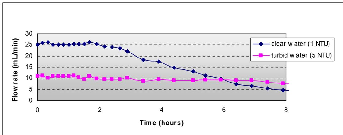
**Figure 5-1:** Experiment on the flow rate of the ceramic filter for water with 2 different turbidities (1 and 5 NTU). The bucket is filled with 10 L of raw water and the flow rate is measured regularly. Due to the decreasing water pressure the flow rate through the ceramic candle filter decreases. As illustrated by the two graphs, the flow rate also depends on the turbidity of the raw water.
