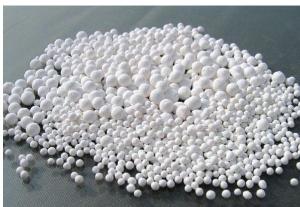
Fig. 7.6 One type of activated alumina: Compalox (Albemarle®)
