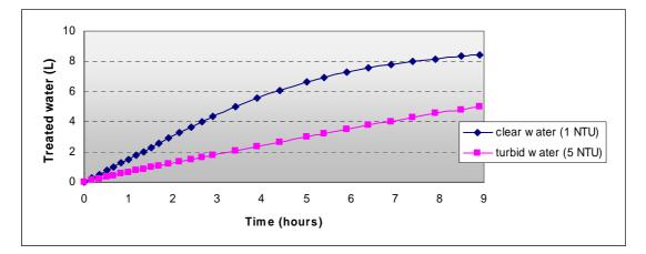
**Figure 5-2:** Experiment on the flow rate of the ceramic filter for water with 2 different turbidities (1 and 5 NTU). The bucket is filled with 10 L of raw water and the amount of treated water measured regularly. After 4 hours 5.6 L of water is filtered for raw water with 1 NTU and 2.4 L of water for raw water with 5 NTU.
