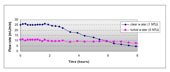
**Figure 5-1:** Experiment on the flow rate of the ceramic filter for water with 2 different turbidities (1 and 5 NTU). The bucket is filled with 10 L of raw water and the flow rate is measured regularly. Due to the decreasing water pressure the flow rate through the ceramic candle filter decreases. As illustrated by the two graphs, the flow rate also depends on the turbidity of the raw water.
