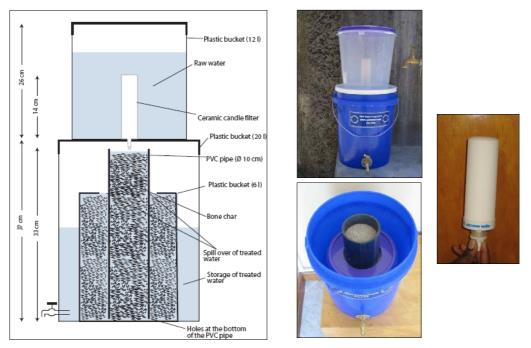
Figure 2-2: Sketch and picture of a combined filter and the ceramic candle.
