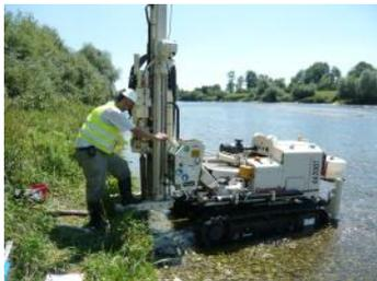
Installation of an observation well (piezometers) on a restored section of the Thur, using a Geoprobe direct-push system.
