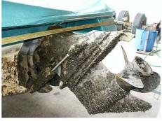
Virtually all of Switzerland's navigable waters are connected via overland boat movements - the thicker the lines, the more frequently the transport routes are used (left). Sterndrive encrusted with zebra mussels (right). (Available for download from the media release at: www.eawag.ch)
