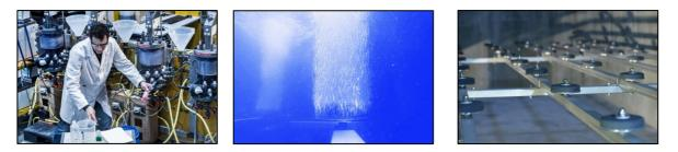
**Picture captions:** Adriano Joss in the Eawag laboratory in Dübendorf. As part of the present EU research project Athene, he has set up 12 sewage treatment plants in laboratory format and is testing whether and how the present biological stage in treatment plants can be optimised for reducing micropollutants (left).
