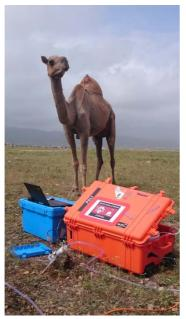
The Mini-Ruedi can quantify numerous gases – currently including helium, argon, krypton, nitrogen, oxygen, carbon dioxide and methane – in environmental systems. Measurements of specific gases can help researchers to understand the underlying processes of gas formation.
