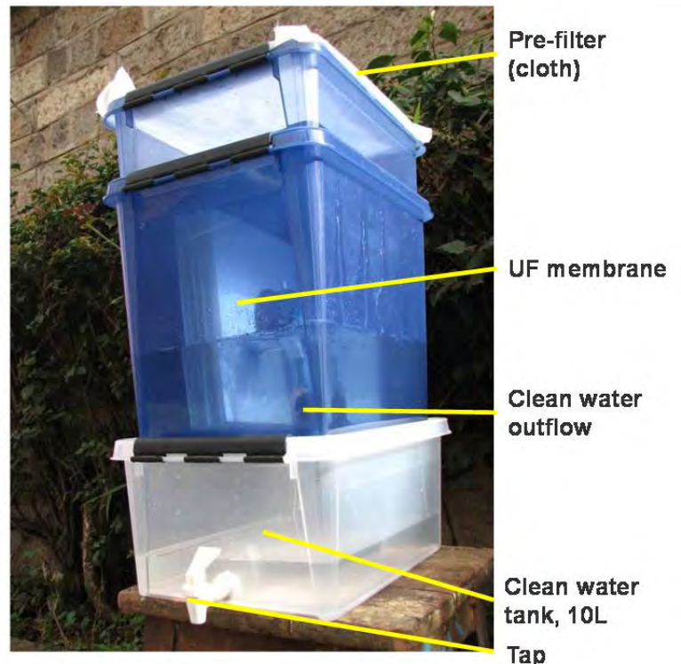
Figure 10 GDM filter prototype \alpha -version for the field study in Kenya (photo: S. Derksen, M. Peter)
