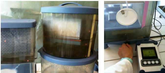
Figure 14 PreSens oxygen spots (red dots) placed in the filters (photo M. Peter and A. Florin)
