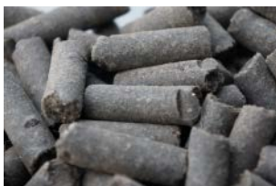
In Senegal and Uganda kilns are heated with pellets made from dehydrated faecal sludge. Photo: Eawag, Linda Strande
