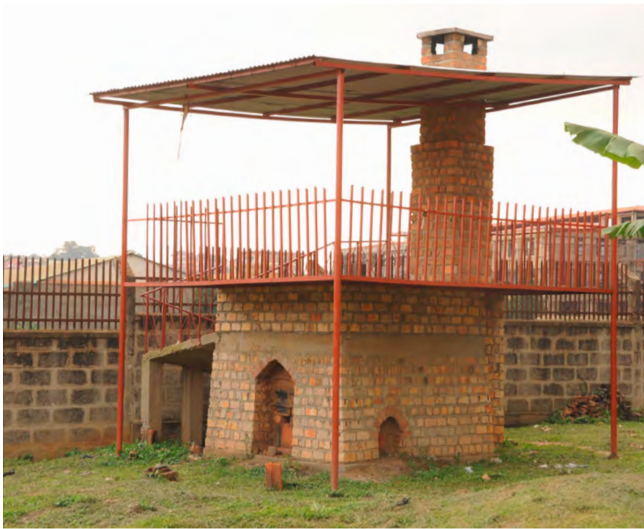
Fig. 6: Pilot-scale kilns fuelled by dried faecal sludge were used for brick production in Kampala (left) and waste oil regeneration in Dakar (right) [10].
