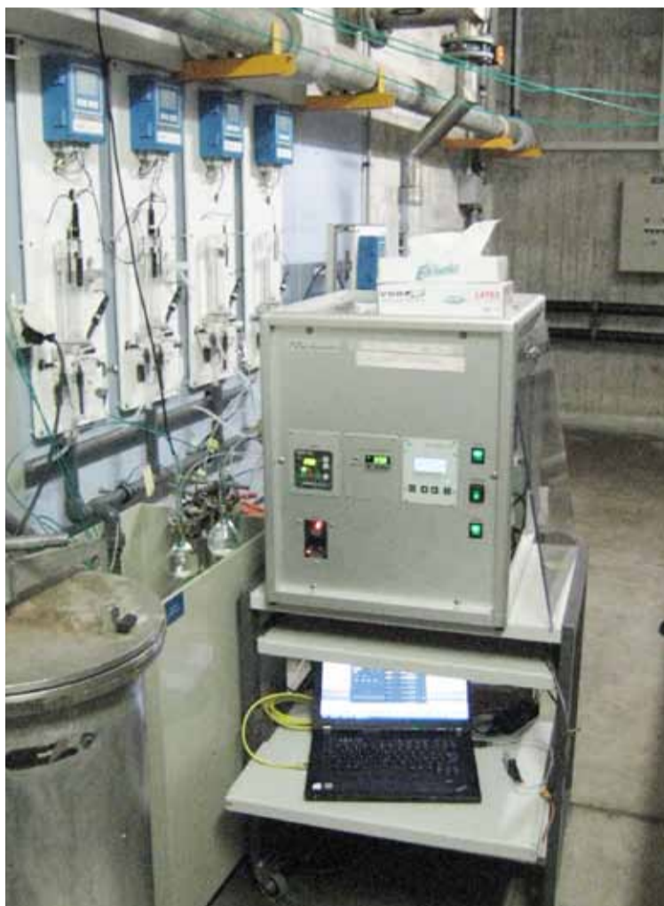
Fig. 2: Equipment used for continuous measurement of trichloramine at various points in the pool water circulation system.
